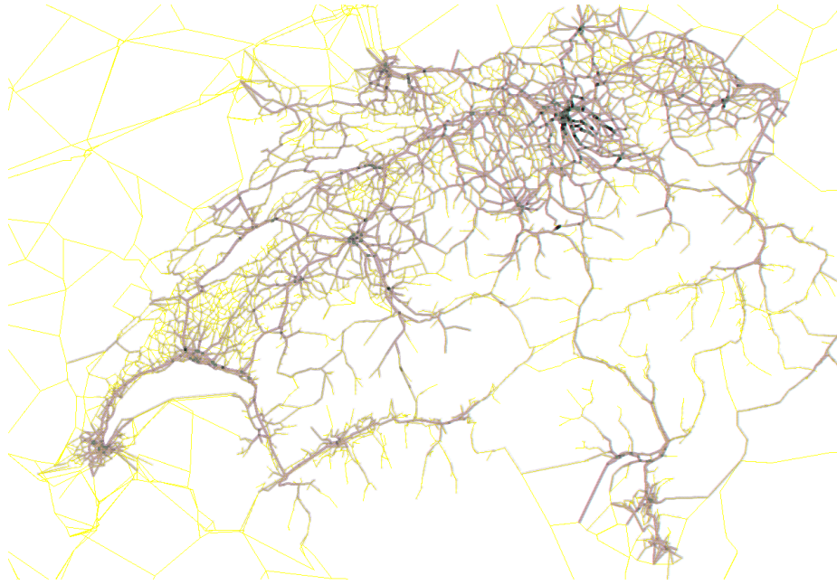
Fig. 4. Most of Switzerland at 8am, simulation result. The graphics shows individual vehicles, but they are so small that they cannot be distinguished. Areas in dark contain traffic jams.
