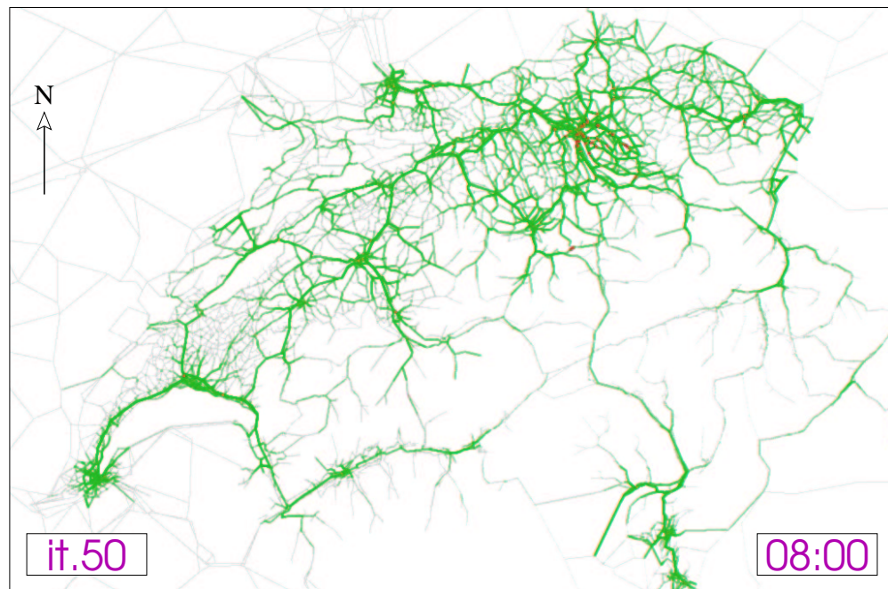
FIGURE 3: Snapshot of Switzerland at 8:00 AM. From the queue micro-simulation, iteration 50.
