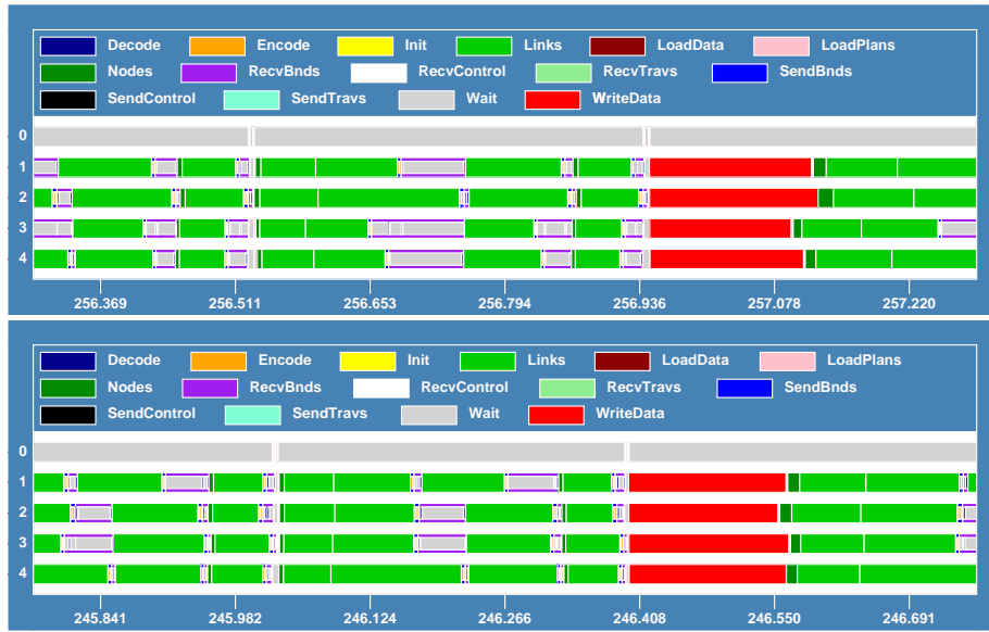
Figure 11: Top : CPU usage without loadbalancing feedback. Bottom : CPU usage with loadbalancing feedback. Note that the idle time, summed over all CPU, is much shorter.
