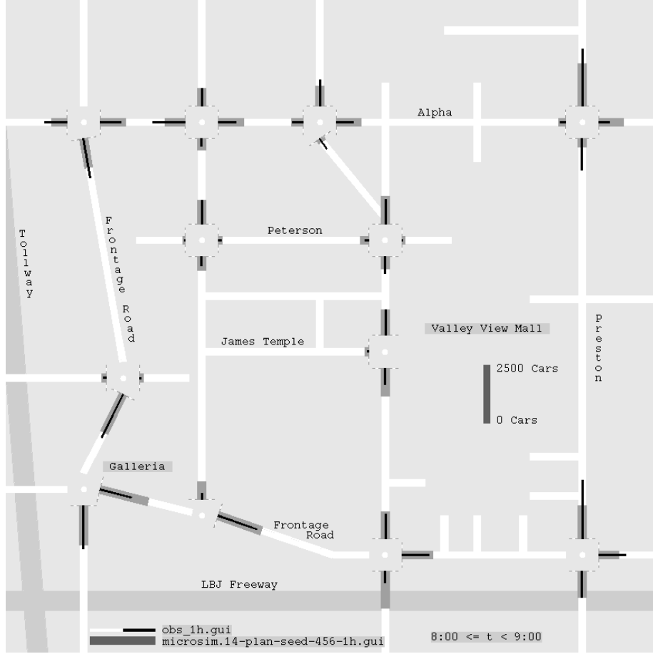
Figure 8: Comparison of approach volumes between simulation result and reality. The lengths of the black bars denote reality; lengths of the gray bars come from the simulation. The data going into this comparison is not entirely consistent, see [67]. From [67].
