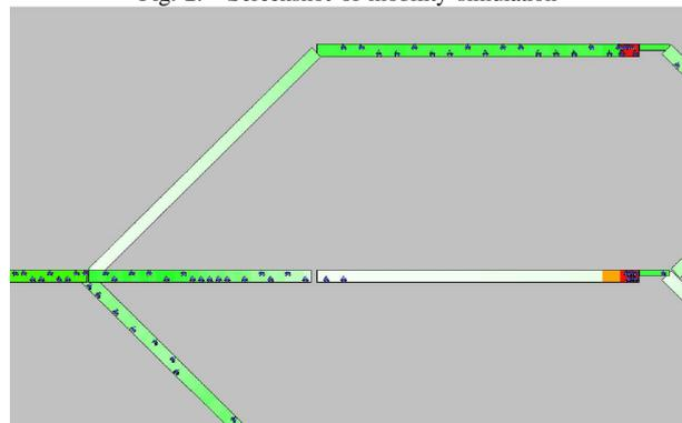
Vehicles move from left to right. At the diverge they choose from one of three routes, each one having a downstream bottleneck. The figure indicates that the macroscopic density (white=none, green=light, red=jammed) is smoothly synchronized with the vehicles' route choice.
