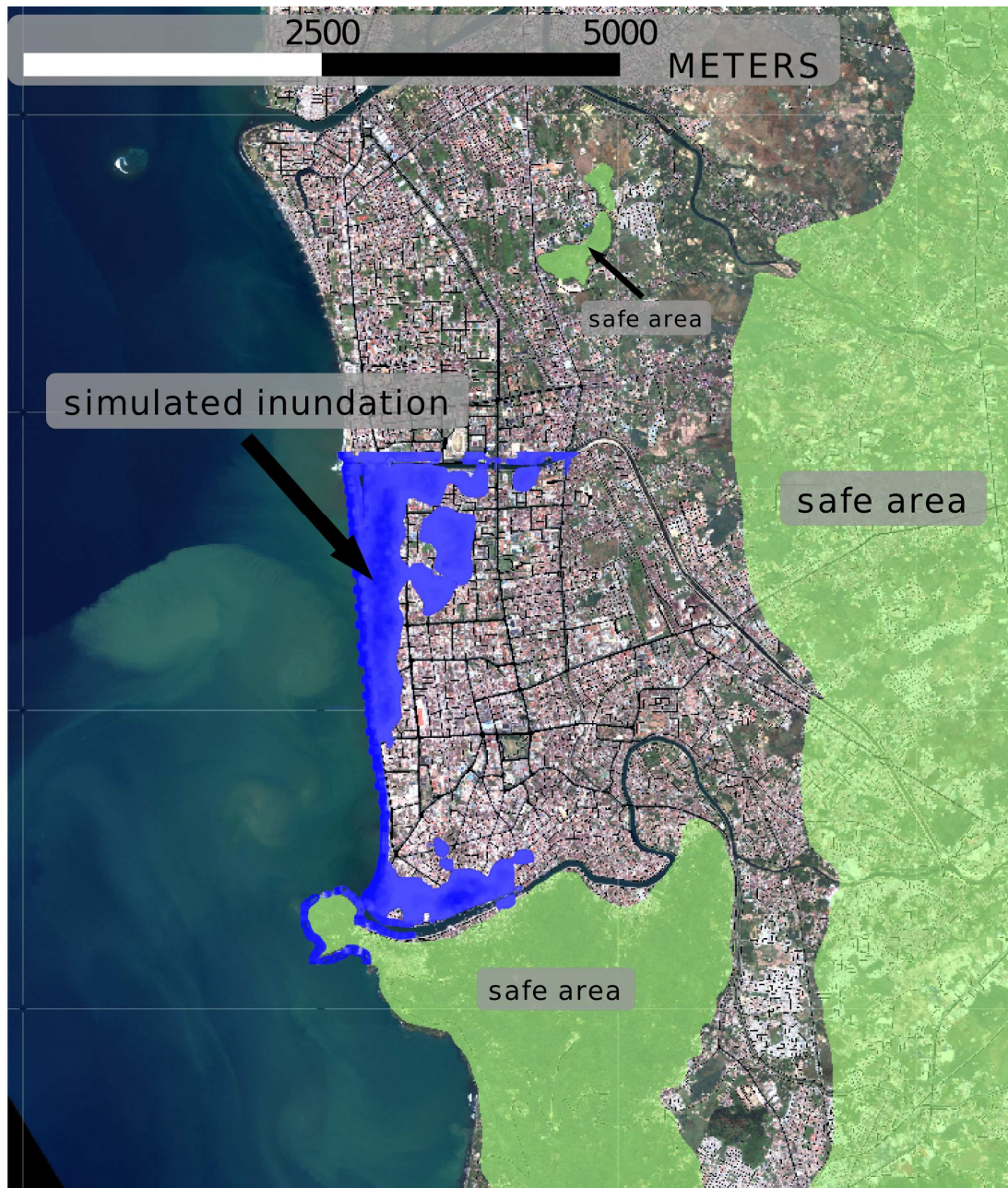
Figure 1: Satellite imagery of the city shows the safe area (light green) and some preliminary results of the flooding simulation (blue area). Satellite imagery by the German Aerospace Center, Oberpaffenhofen (2007)
