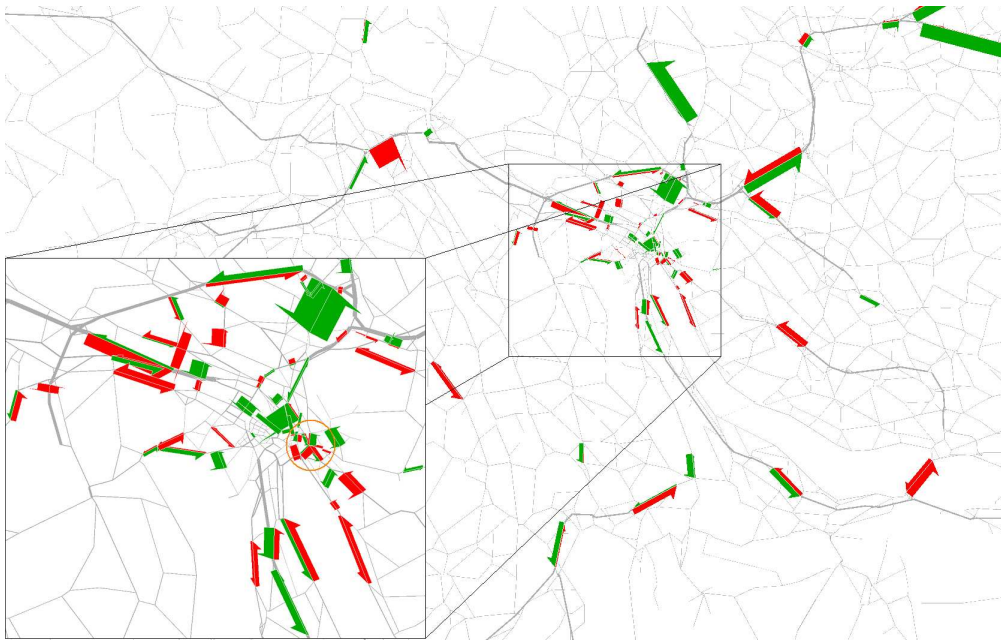
Figure 1: Spatial layout of the link-based utility offsets at 8 am–9 am. Red: Counts are too high, negative utility offsets try to discourage traffic. Green: Counts are too low, positive utility offsets try to encourage additional traffic. Width corresponds to the magnitude of the utility offset.
