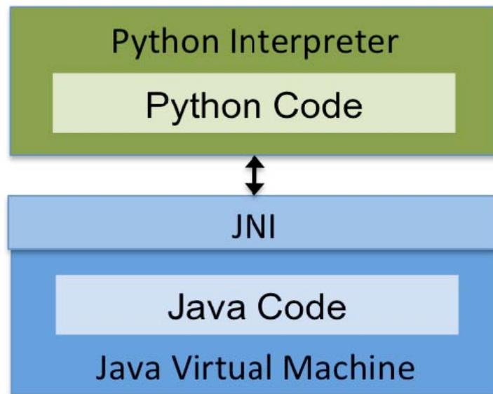
Figure 4: Communication between CPython and the Java Virtual Machine via JNI.
