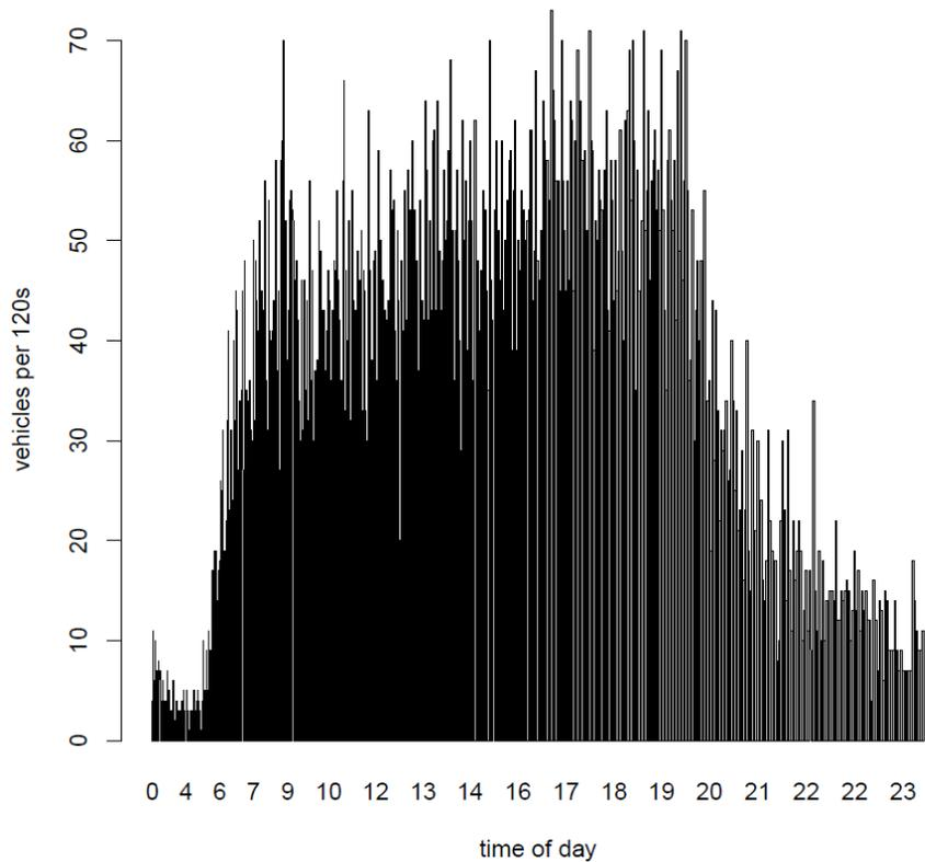
**Figure 1: Inflow of vehicles onto the test road over time of day in 120 seconds intervals for July 07<sup>th</sup> 2009.**
