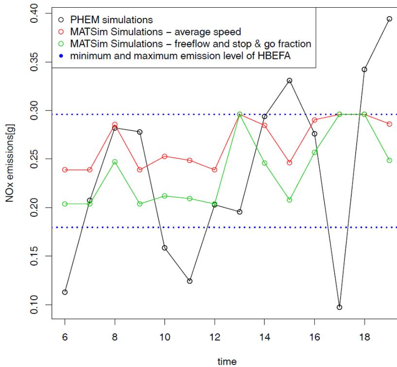
Figure 4: NO<sub>x</sub> emission levels (diesel) for July 07<sup>th</sup>, 2009: in black PHEM data, in color the two MATSim-based approaches.
