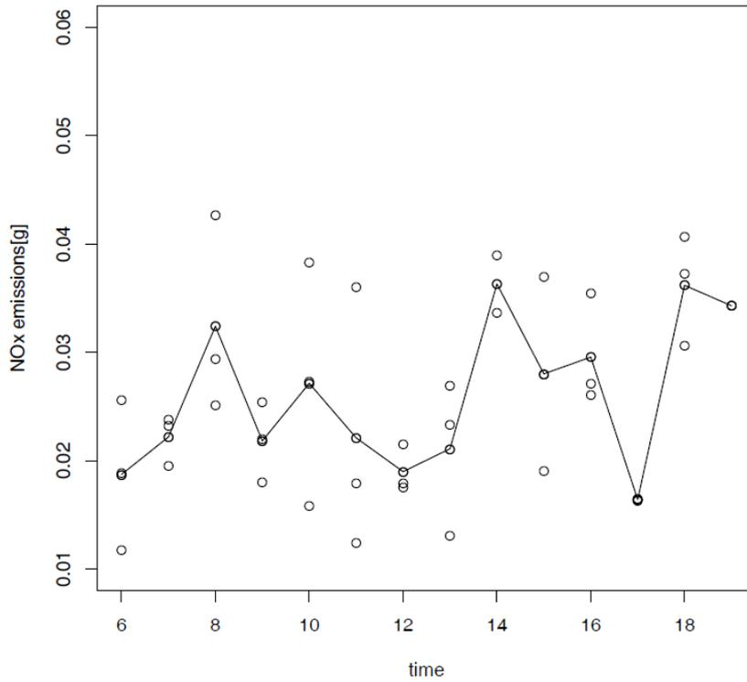
Figure 3: NO<sub>x</sub> emission levels (gasoline) based on PHEM; average over three days.
