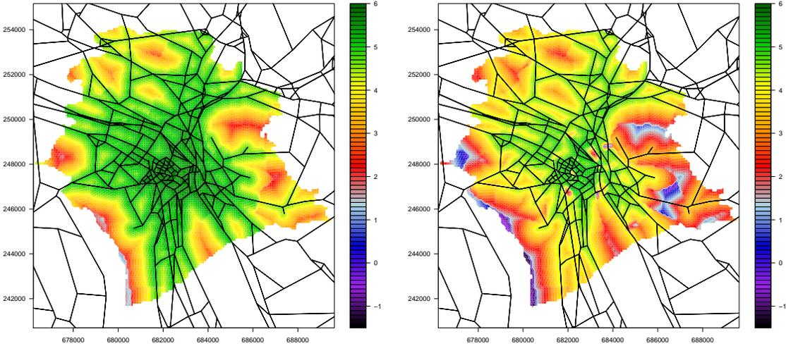
(a) Free speed car travel times in accessibility computation (b) Congested car travel times in accessibility computation (reference setting)
