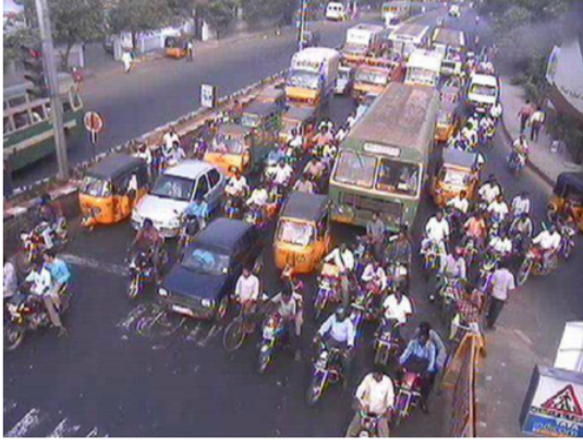
(a) Seepage of smaller vehicles at traffic signal [6].
