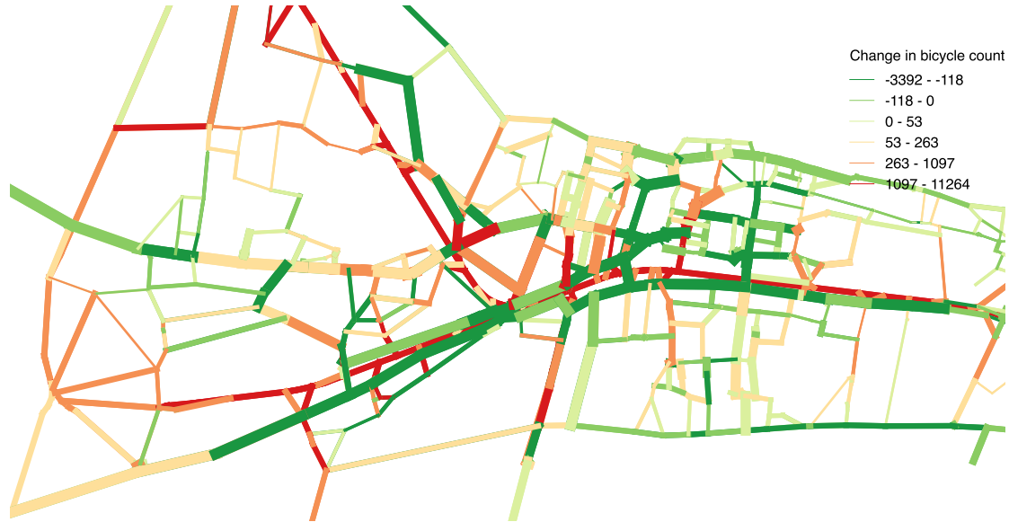
Figure 5: Change in bicycle count for business-as-usual scenario with respect to BSH-b policy scenario (green and red colors represent a decrease and increase in bicycle traffic respectively). Thicker lines represents higher capacities of links (.e.g arterials).
