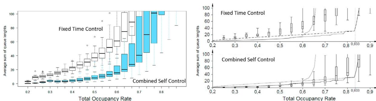
Fig. 5. Simulation results for stochastic arrival times: MATSim (left), MATLAB simulation by Lämmer<sup>2</sup> (right)
