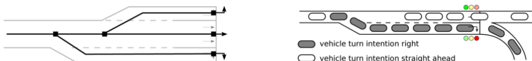
Fig. 1. Links with multiple lanes in MATSim. Each lane is represented by its own FIFO queue. Traffic signal control for different turning moves is captured. Vehicles on different lanes can pass each other, unless the queue spills over. Source: Grether and Thunig (2016).
