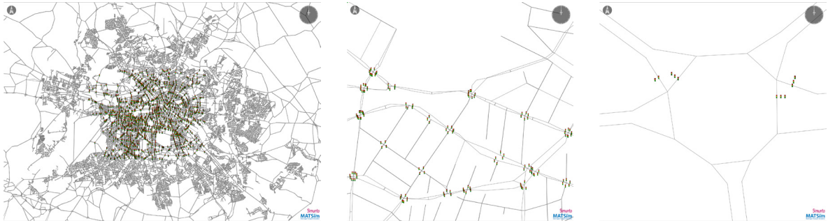
Fig. 7. Different network extracts of the Open Berlin Scenario with traffic signals and lanes. Left: City of Berlin and all generated signal locations (lying within a bounding box including the inner city); Middle: Region around the zoological garden – exemplary shows the correctness of signal locations; Right: Signalized roundabout of Großer Stern, visualizing one of the issues of the approach discussed in Sect. 5.
