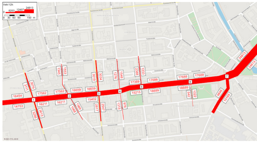
Fig. 5. Traffic load constructed from counts in the study area along Leipziger Straße, Berlin, Germany.
