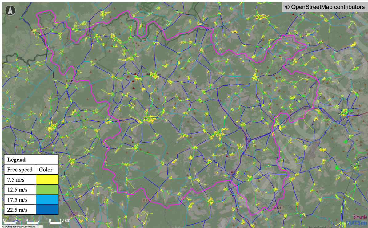
Figure 4: Modelled road network: the free speeds of road segments are indicated by the color
