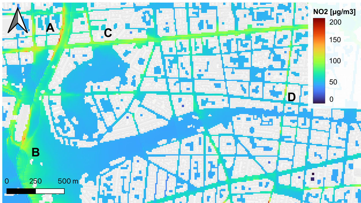
Figure 8: \text{NO}_2 concentrations on a continuous scale. The area depicted corresponds to the rectangle in figure 6b. Effects of the building layout as well as the street layout are highlighted by letters A - D
