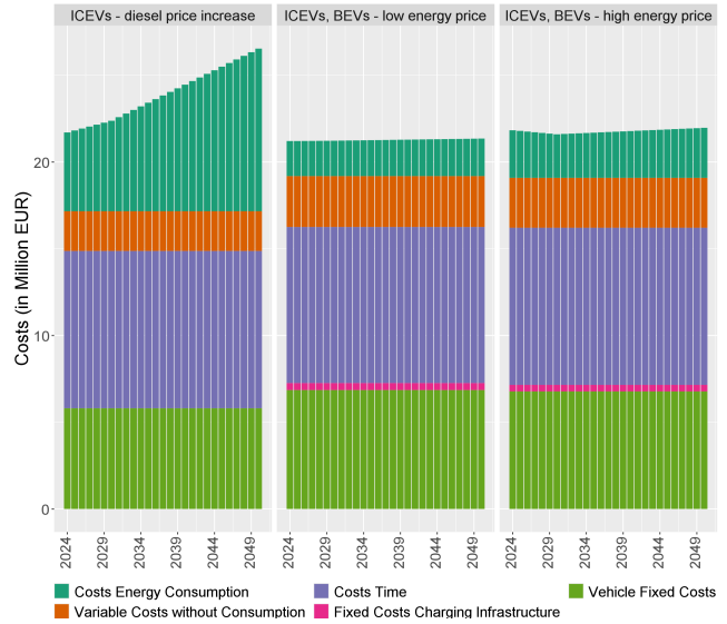
Fig. 4: Annual costs per cost type. The results are based on the most cost-effective solution fleet for a scenario in year 2024 and an assumed energy price for the following years.
